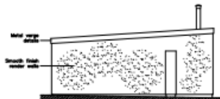
Commercial garage - Existing west elevation SCALE 1:100
