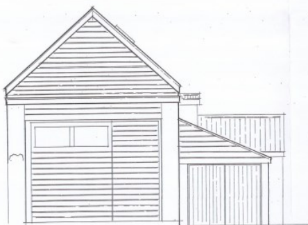
FRONT ELEVATION facing main house elevation and doors timber boarding finish
