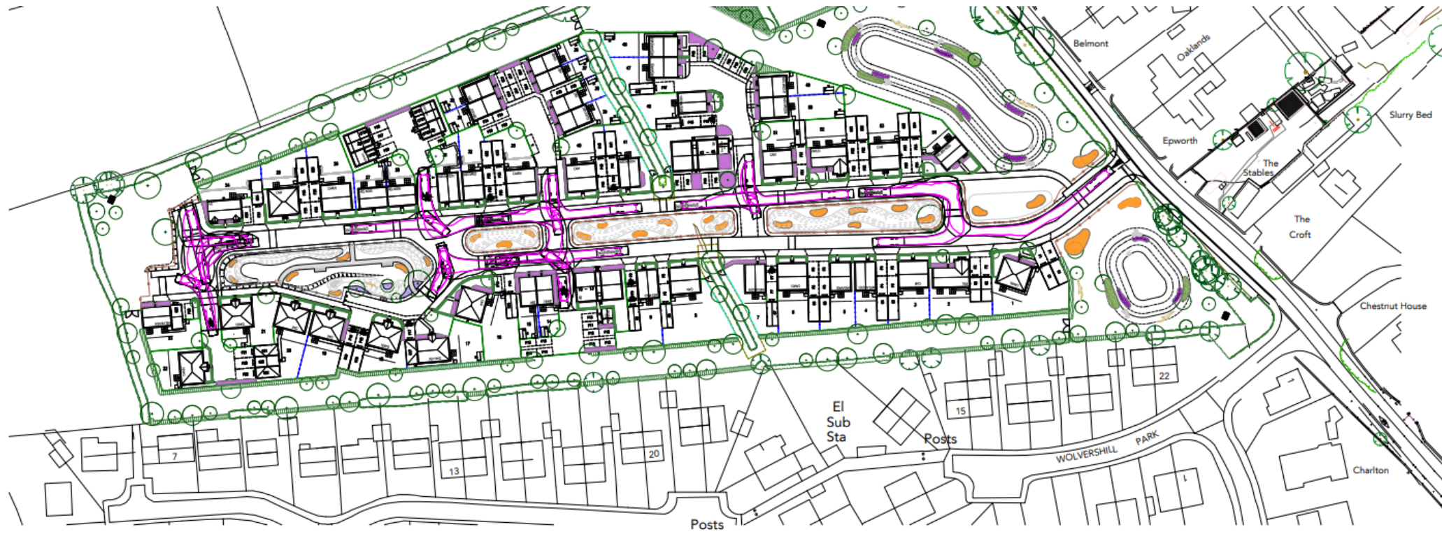
REFUSE VEHICLE TRACKING LAYOUT @ 1:500
