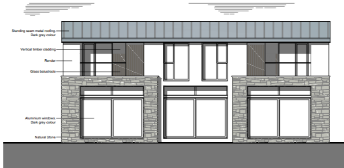
Rear Elevation South Facing
