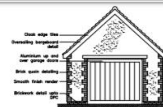
Detached garage - Proposed east elevation
