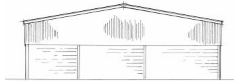
END NORTH Yorkshire boarding over blockwork walls
